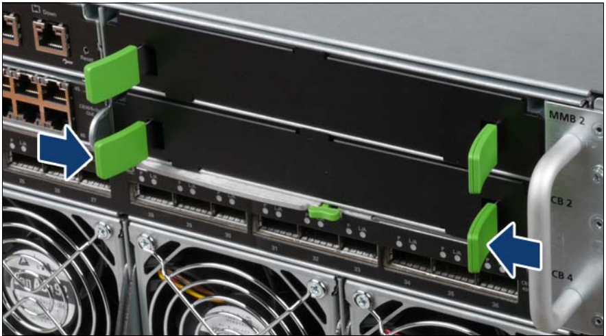
Figure 36: Removing a dummy connection blade module
